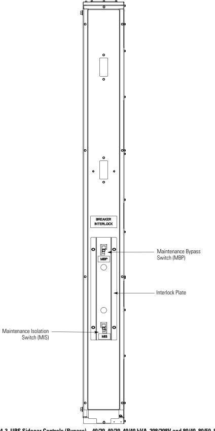
Figure 4-3. UPS Sidecar Controls (Bypass) – 40/20, 40/30, 40/40 kVA, 208/208V and 80/40, 80/50, 80/60, 80/80 kVA and 120/100 and 120/120 kVA, 480/480V with MBP and MIS
